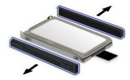
7. Attach the side rubber rails to the new hard disk drive or the side spacer rails to the new solid state drive.
